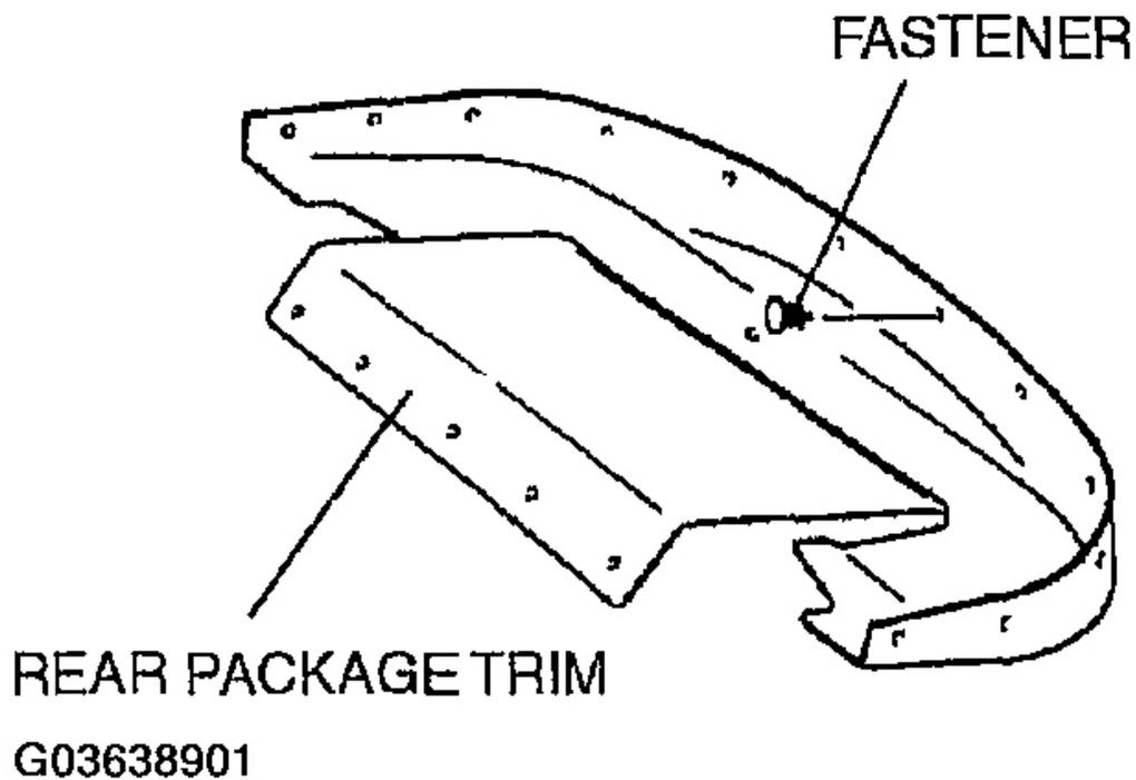
**Fig. 15: Removing Rear Package Trim**
