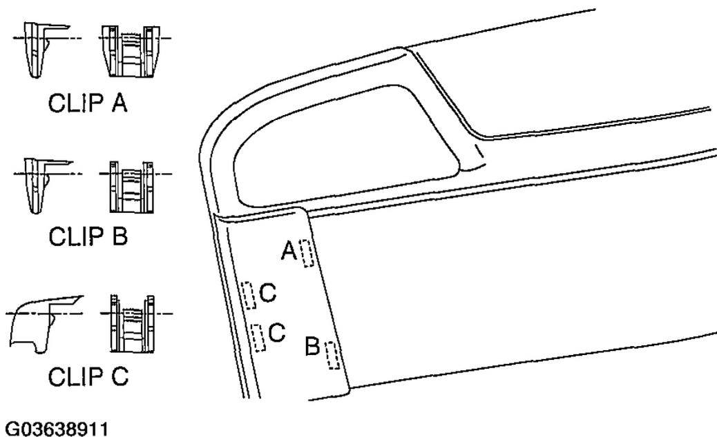
**Fig. 25: Removing Belt Cover**
