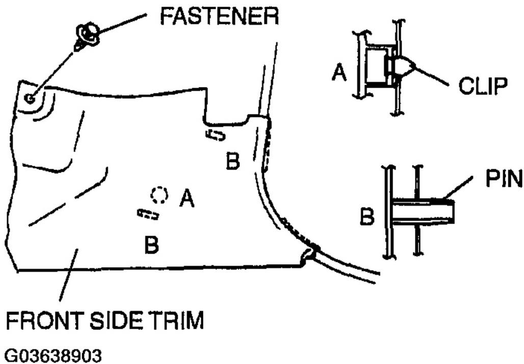
**Fig. 17: Replacing Front Side Trim**
