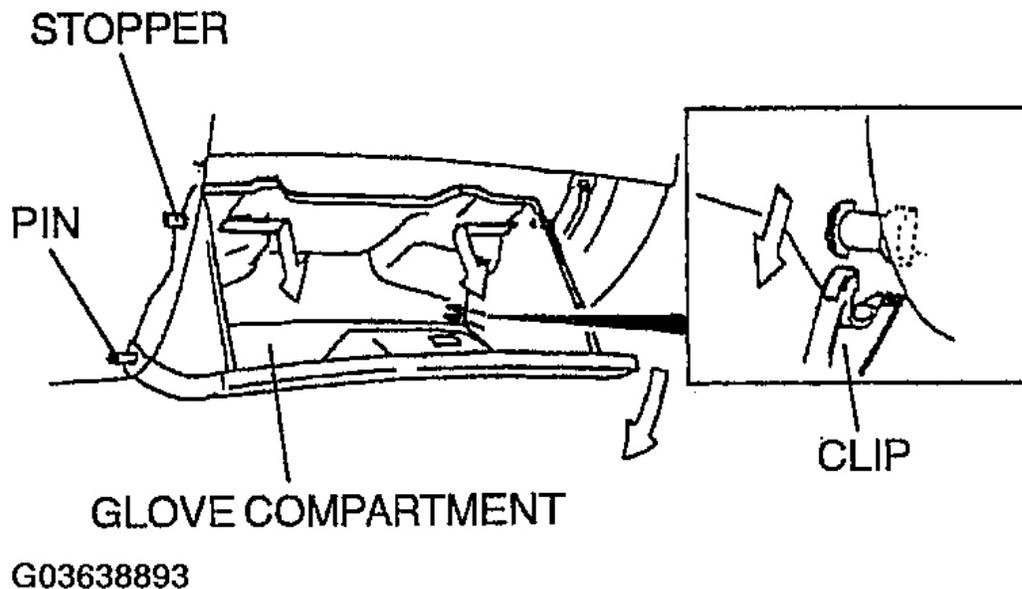
**Fig. 7: Removing Glove Compartment**
