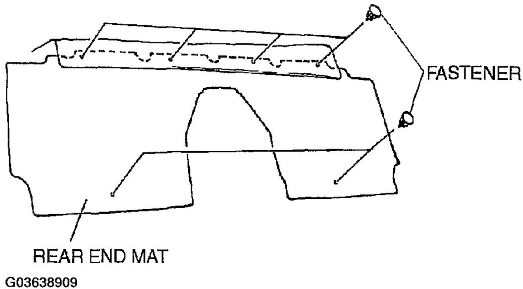
**Fig. 23: Removing Rear End Mat**
