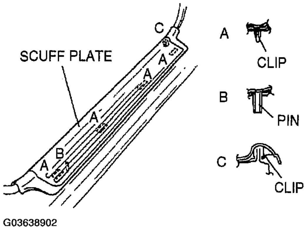
**Fig. 16: Replacing Scuff Plate**
