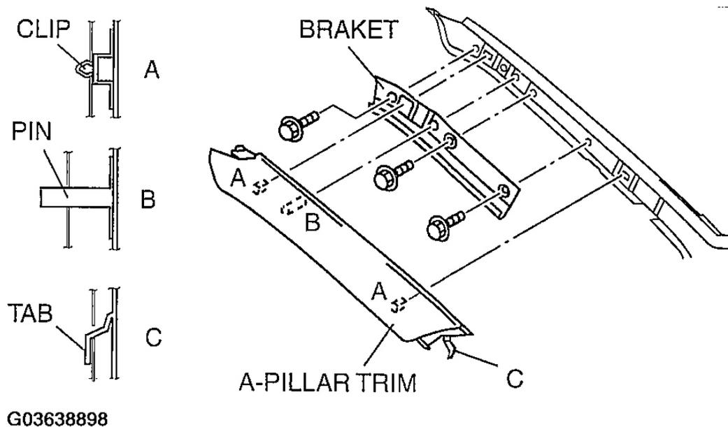
**Fig. 12: Removing A-Pillar Trim**
