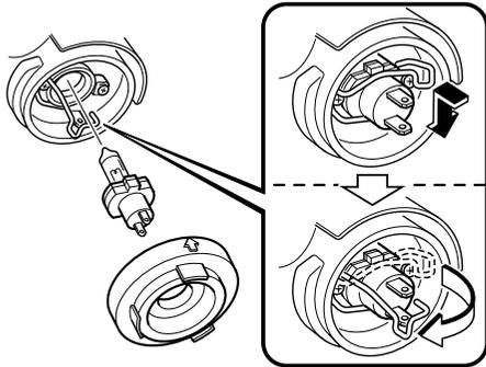
7. Swing the retaining spring out and away to free the headlight bulb.
