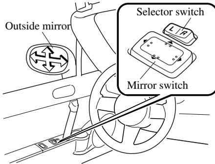
After adjusting the mirror, lock the control by placing the selector switch in the middle position.
