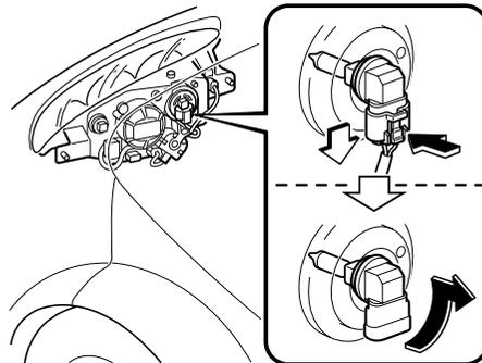
3. Install the new socket and bulb assembly in the reverse order of removal.
