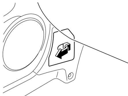
3. Pull the fuse straight out with the fuse puller provided on the inside of the engine compartment fuse block cover.
