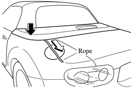
6. Lightly move the deck and verify that it is secured completely.
