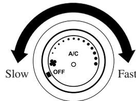
Turn the dial to adjust to the desired fan speed.
