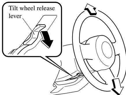
After adjusting, push the wheel up and down to be certain it's locked before driving.
