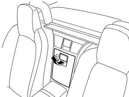
To open the fuel-filler lid, pull on the remote fuel-filler lid release.
