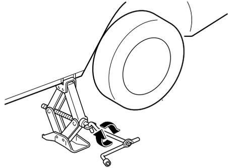
5. Remove the lug nuts by turning them counterclockwise, then remove the wheel.
