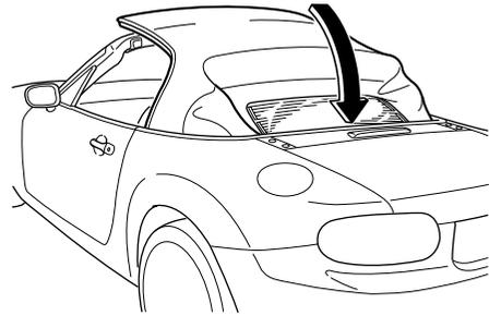
8. After the convertible top has been folded down, press the back end of the folded down convertible top until a click sound is heard, then the front end. Lightly rock the retracted convertible top to make sure it is securely locked.
