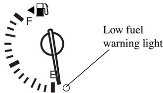
This warning light signals that the fuel tank will soon be empty. Refuel as soon as possible.
