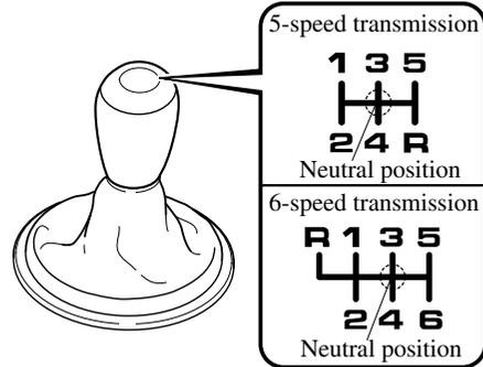
The vehicle is equipped with either a 5-speed or 6-speed manual transmission. The shift pattern for each is shown above.
