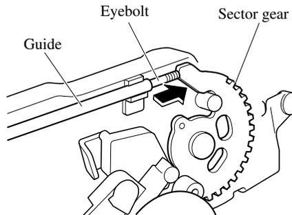
10. Press and rotate the sector gear rearward to release the lock.
