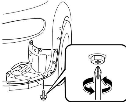
3. Turn the center section of the plastic retainers counterclockwise and remove them, then remove the mudguard.
