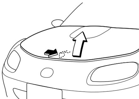
3. Grasp the support rod in the padded area and secure it in the stay hole indicated by the arrow to hold the hood open.
