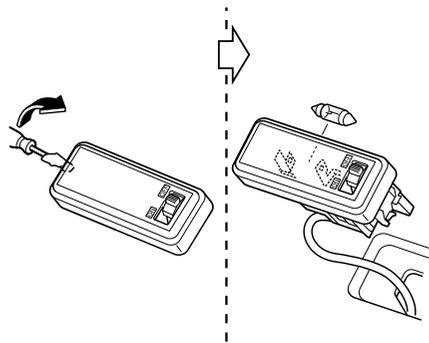
3. Install the new bulb in the reverse order of removal.
