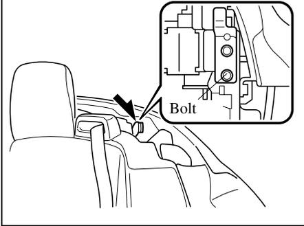
3. Use the eyebolt to get enough torque on the short leg of the Allen wrench and turn the Allen wrench 4 times counterclockwise.
