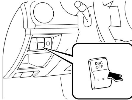
Press the switch again to turn the TCS/DSC back on. The DSC OFF indicator light will go out.
