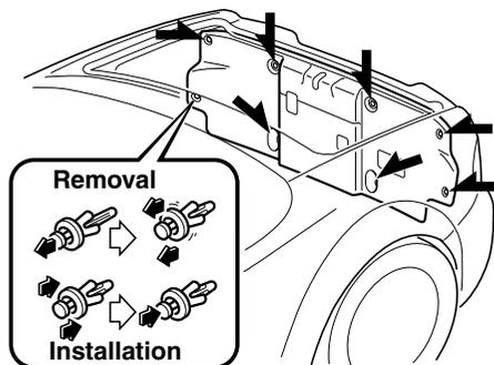
2. On the side the bulb is to be replaced, pull the center section of the plastic retainers and remove them, then remove the trunk side trim.
