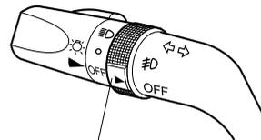
To turn them off, rotate the fog light switch to the OFF position or turn the headlight switch to the
