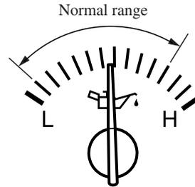
Engine oil pressure is normal when the engine oil pressure gauge needle points within the normal range.
