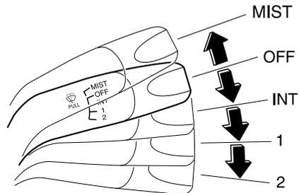
Turn the wipers on by pulling the lever down.
