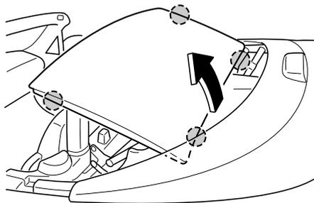
3. Grasp the hardtop along its side surface and the rear area of the rear glass, pull the hardtop towards the front of the vehicle, and completely close it.
