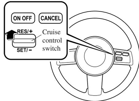
Your vehicle has a tap-up feature that allows you to increase your current speed in increments of 1.6 km/h (1 mph) by a momentary tap of the cruise control switch. Multiple taps will increase your vehicle speed 1.6 km/h (1 mph) for each tap.
