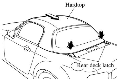
13. Lift the hardtop straight off the body to prevent damage to the rear deck latches and studs.
