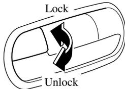
To lock any door with the door-lock knob from the outside, push the door-lock knob to the lock position and close the door.
