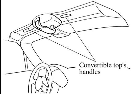
6. Sitting in a seat, grasp the convertible top's handles, and press the convertible top against the windshield. Move the top latch slowly to make sure the anchor engages with the striker, then rotate the top latch to the lock position until a click sound is heard.
