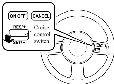
Your vehicle has a tap-down feature that allows you to decrease your current speed in decrements of 1.6 km/h (1 mph) by a momentary tap of the cruise control switch. Multiple taps will decrease your vehicle speed 1.6 km/h (1 mph) for each tap.
