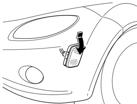
2. Turn the socket and bulb assembly counterclockwise and remove it.
