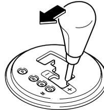
To return to automatic shift mode, shift the lever from M to D.
