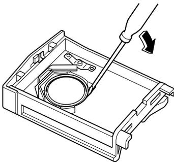
5. Put in the new battery (CR1620 or equivalent) with the positive pole (+) facing down.
